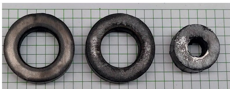
Fig. 3 Sintering of MgB_2 sintered with FAST-SPS [3, 4], courtesy of Daniel Wilkinson
