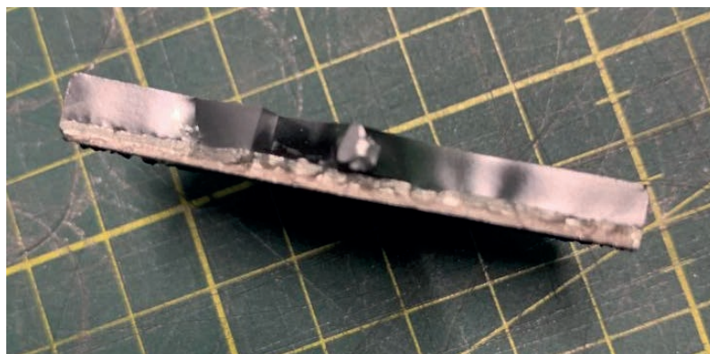
Fig. 11 Graded material – W/ B_4C – B_4C [2, 3]. A layer of B_4C (dark layer on top) was combined with a layer of mixed B_4C/W and a layer of pure W (copper colour at the bottom). This resulted in a good bond
