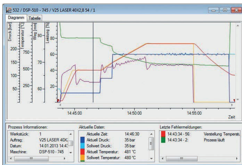
Fig. 2 A typical sintering cycle for metallic materials [2]
