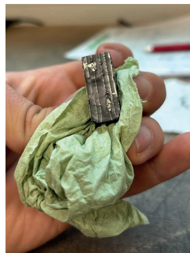
Fig. 12 Laminated composite design with B_4C and W [2, 3]
